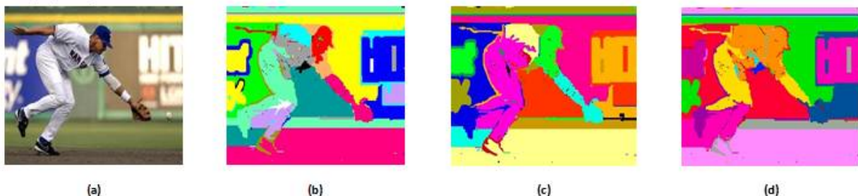
Fig. 5. Sub image (a) shows an Input Frame of a sports video sequence. The different segmentation outputs obtained on this frame for (b) K = 300, (c) K = 900, (d) K = 1200.
